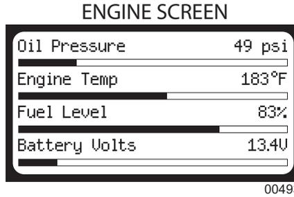
Additional information may be viewed while the unit is in Manual or Auto mode. By pressing the Page Select button, the operator will select one of the following screens; Running screen, Password screen, or History screen. In each of these page selections the operator may press the ▲ or ▼ buttons to display additional information as follows:
