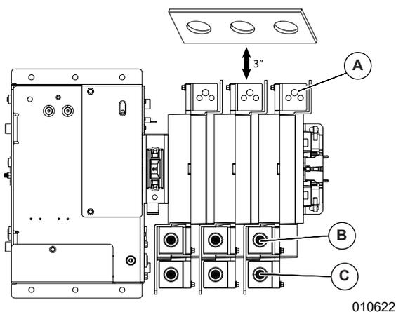
**Figure 3-3. Typical 3-Pole Transfer Mechanism (200 Amp Shown)**
