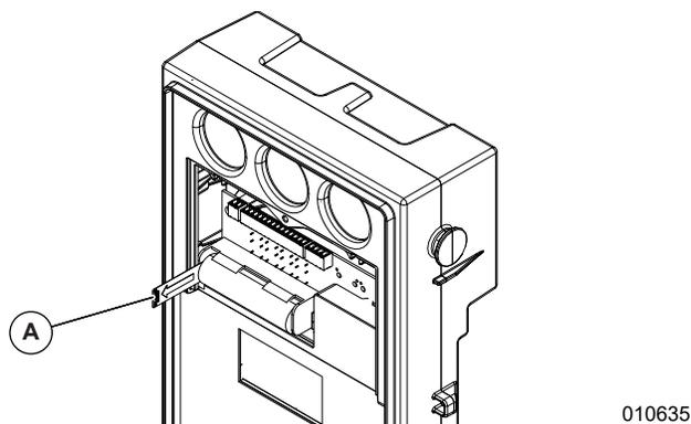
**Figure 4-5. Remove Battery Isolation Tab**
