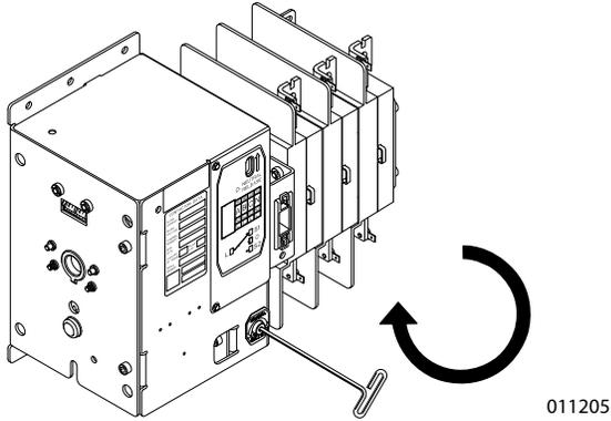
**Figure 4-3. Rotate Manual Operator Clockwise**
