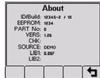
**Note:** This screen can not be exited until the checksum calculation is complete. Checksum calculation takes approximately 10 seconds and is complete when the checksum value changes from Calculating... to a hexadecimal value such as 0x704E – OK.
