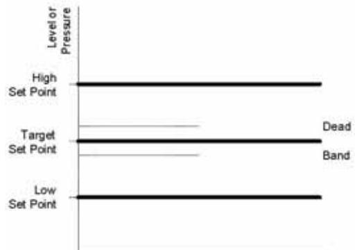
**Note:** The dead band entered is the amount above and below the target point. For example, if the target is 5.0 ft (1.52 m) with a 0.1 ft (.03 m) dead band, the dead band is 4.9 to 5.1 ft (1.49 to 1.55 m).
