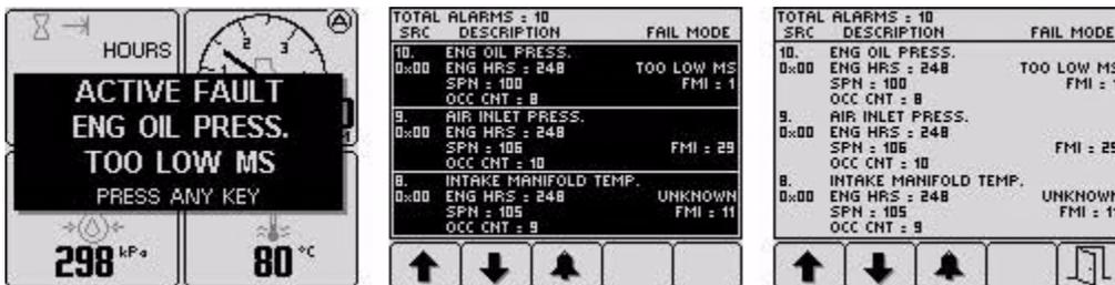
In the examples above are alarm list screens showing unacknowledged conditions and acknowledged alarms. After acknowledgement, the exit button becomes active.
