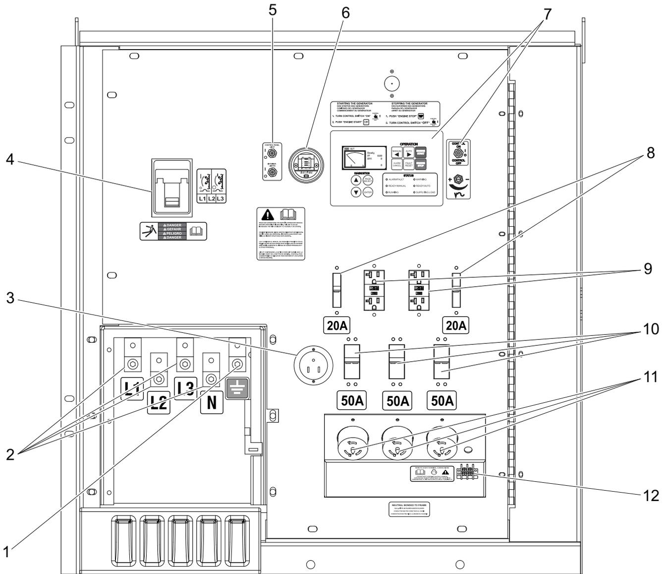
1. **GENERATOR GROUND CONNECTION LUG:** This lug is for connecting a good earthen ground per any local, state or National Electric Code (NEC) guidelines before starting the generator.
