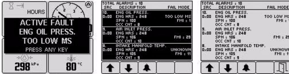
Example alarm message, alarm list screens showing unacknowledged conditions and acknowledged alarms. After acknowledgement, the exit button becomes active.
