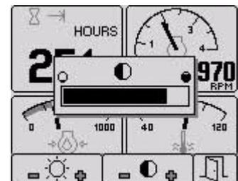
**Note:** *The display adjusts the contrast with ambient temperature. Manual contrast adjustments are only necessary with extreme climate change.*
