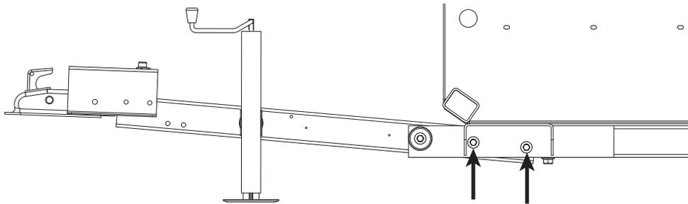
**Note:** If the jack was used to support the unit while removing the shipping brace, the jack must be moved back to the tongue location before the unit can be towed. Connect the trailer tongue to a vehicle or other support and move the jack to the tongue location.
