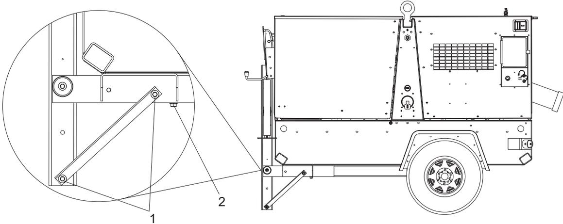
3. Remove the shipping brace and slide it into the trailer tube opening. Secure the brace to the trailer with the bolt located on the underside of the trailer (2) and a new nylon locking nut.
