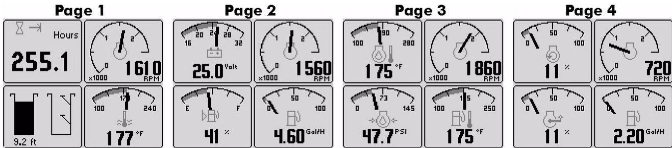
**Note:** Engine Hours are displayed as a digital value even on Analog Gauge Pages. The default gauge pages represent 13 selections since the tachometer is repeated in the upper right quadrant of each page.
