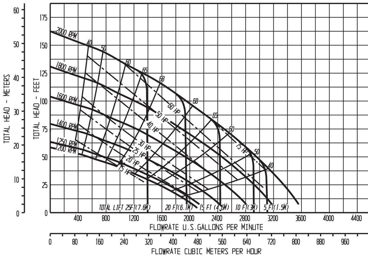
**Note:** Performance includes losses for check valve, priming system and open clearance wear ring.
