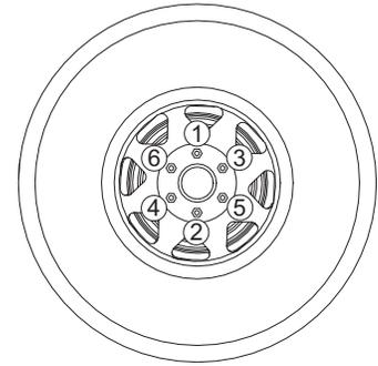
After the first road use, retorque the lug nuts in sequence.
