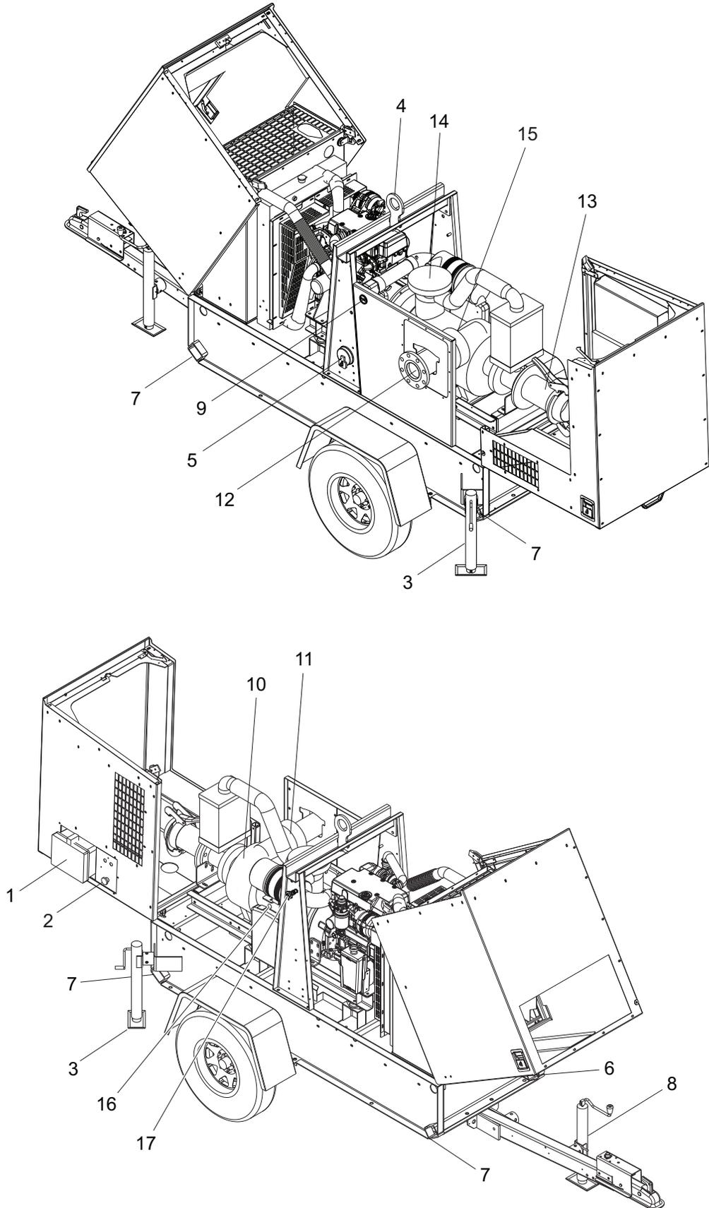
1. **CONTROL PANEL.** Controls and indicators for pump operation.
