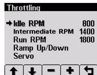
compensate for parasitic loads such as hydraulic pumps or compressors. Idle RPM is the low speed setting of the optional two state or three state throttle switches.
