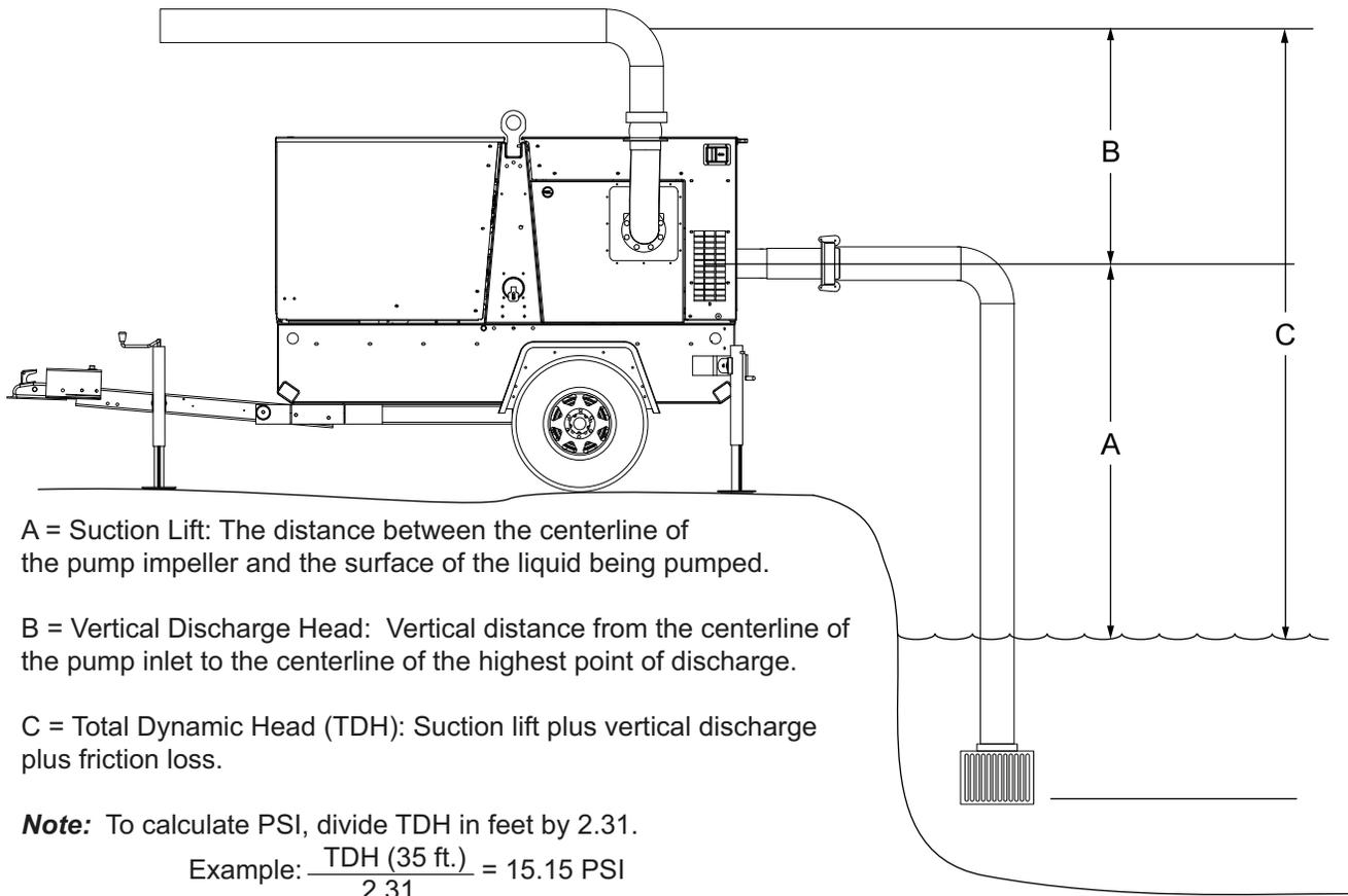
A = Suction Lift: The distance between the centerline of the pump impeller and the surface of the liquid being pumped.
