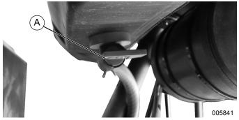
Figure 3-2. Fuel Shut-Off Valve
