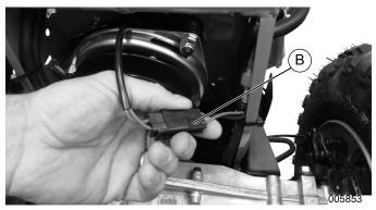
Figure 4-9. Clutch Connector
