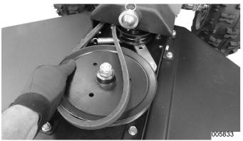
Figure 2-7. Install Belt on Spindle Pulley
