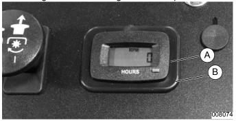
Figure 2-13. Maintenance Meter Installation
