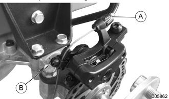
Figure 4-16. Brake Cable Adjustment
