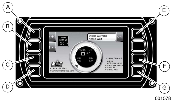
Figure 2-5. Controller in AUTO Mode
