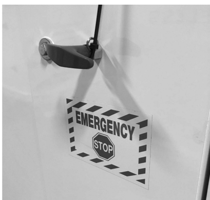
Figure 3-11. Emergency Stop T-Handle
