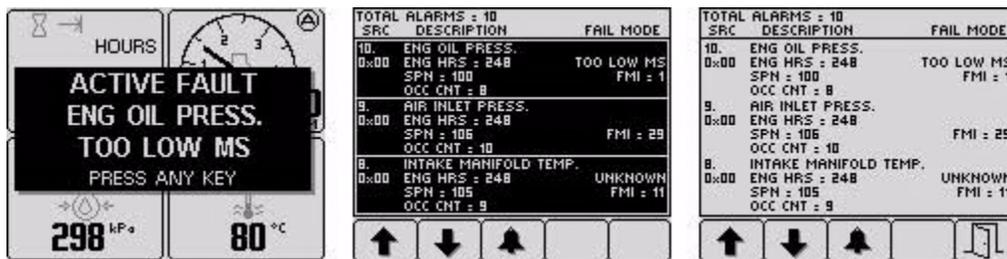
In the examples above are alarm list screens showing unacknowledged conditions and acknowledged alarms. After acknowledgement, the Exit button
