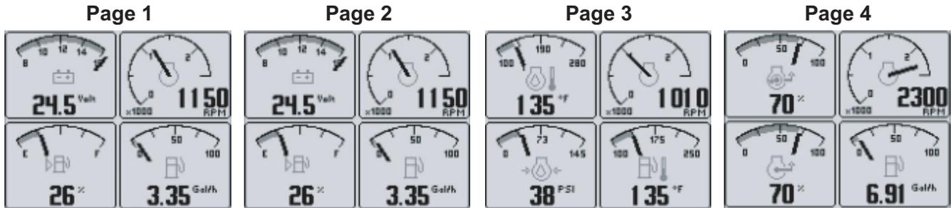
**Note:** Engine hours are displayed as a digital value even on Analog Gauge Pages. The default analog gauge pages represent 13 selections since the tachometer is repeated in the upper right quadrant of each page.
