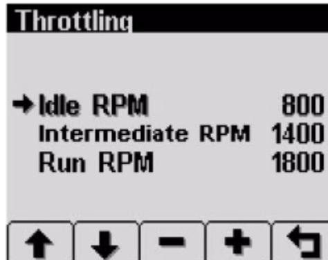
The “Throttling” menu allows programming the automatic start/stop throttle profiles.
