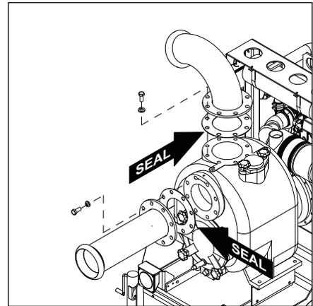
4. Attach a rigid hose to the intake (suction) side of the pump. To prevent cavitation, the suction hose/piping should be at least as large as the pump flange, never smaller. The pump should be at the highest point of the hose/piping. All suction piping and fittings should be checked for any foreign material (rocks, bolts, wire, etc.) and also any sharp burrs that could disrupt the flow. Make sure the O-ring seal is present in the fitting on the pump before attaching the fitting.
