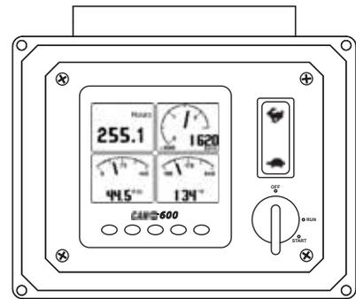
If the ECU is preheating when the key switch is turned to the “RUN” position, a Preheat screen will appear. Preheat time varies with atmospheric and engine conditions. After waiting for the Preheat screen to extinguish, the engine is cranked by turning and holding the key switch in the “START” position until the engine starts.
