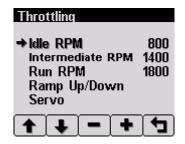
**Note:** The minimum engine speed is set by the ECU. Requesting a lower speed causes the engine to run at the ECU minimum speed. RPM limits are programmed into the panel to limit the requested speed. Changing the panel Minimum Requested RPM and Maximum Requested RPM requires using the CANplus Configurator.
